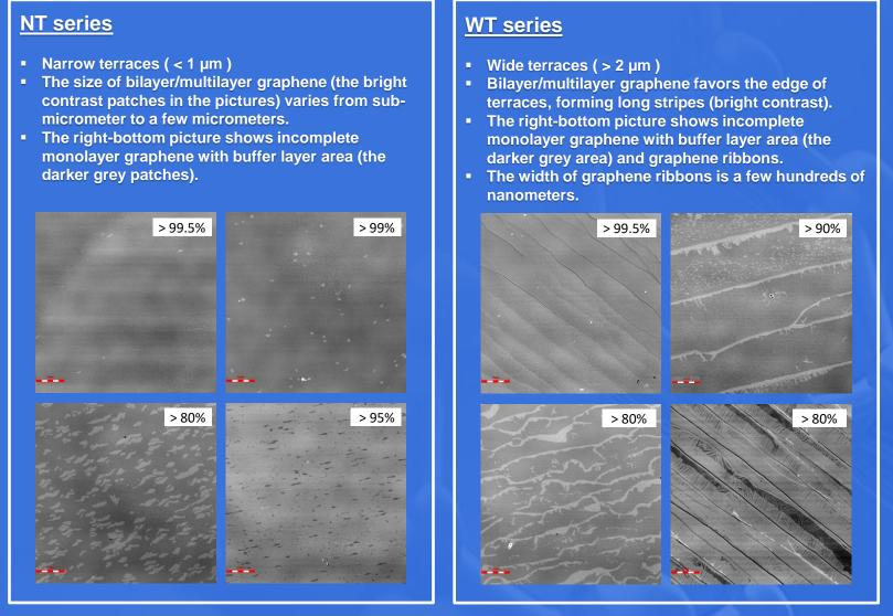
\* Images of graphene on silicon carbide with different monolayer coverage rates (indicated in the upper right corner of each image). The scale bar is 10 µm.
