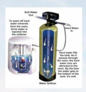
Softening plants is designed to cater to the requirement of scale prevention of Utility / Plumbing Fixtures from total hardness. Softeners are available for Bungalow/ Institutional/ Industrial applications.
