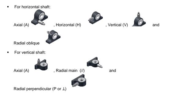
\*\*\*\* Sensor position picture: it is possible to replace the pictogram by a picture of the sensor:
