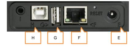
Those connectors are behind a trapdoor. It must remain close in industrial environment to preserve the IP65 protection. Use those connectors only in office environment.
