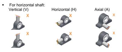
• For horizontal shaft and Axial (A), Radial oblique 1 (1) and Radial oblique 2 (2) directions
