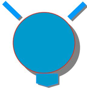
When a bearing is equipped with radial sensors set 90° apart from each other, it is possible to plot the orbit representing the path of the measured element in the plane defined by the two sensors.
