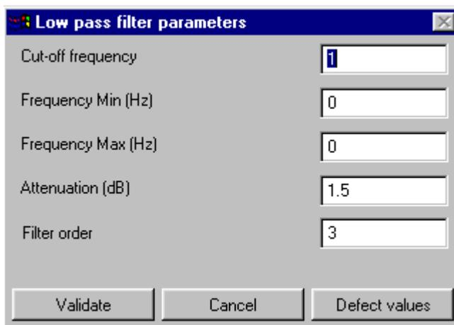
The 'Cut-off frequency' field is for Low-pass and High-pass filters. It is not accessible for Band-pass and Band-stop filters.
