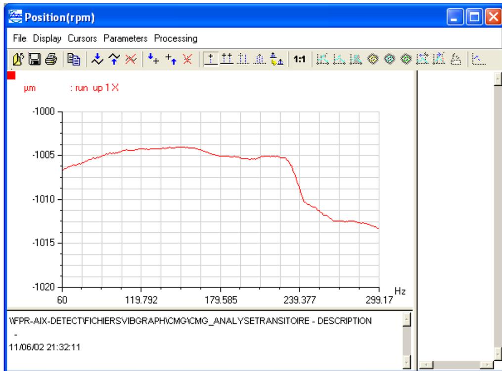
The Position(rpm) representation describes the shaft position in the X or Y measurement plane versus rotation speed.
