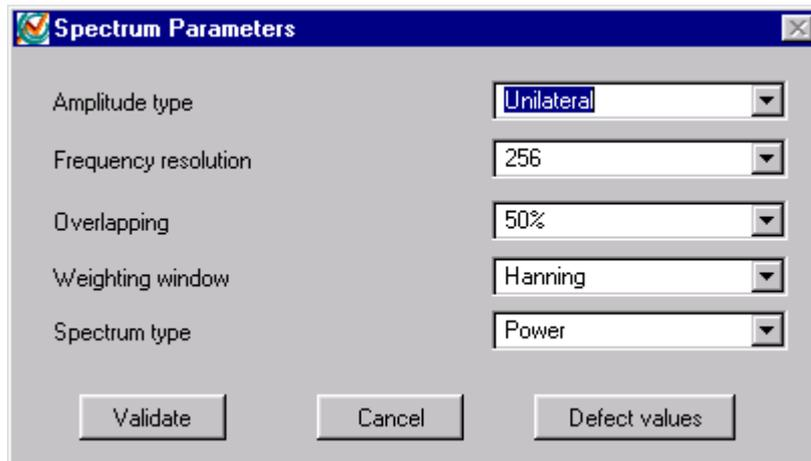
This processing computes various types of spectra starting from a time signal. The algorithm is based on the Welch method:
