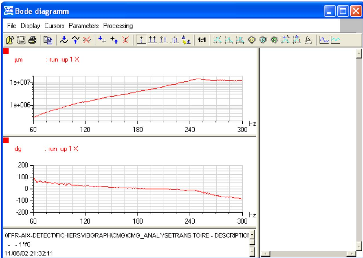
On a Bode diagram, a critical speed can be detected by a local amplitude maximum or by an inverse phase inflection.
