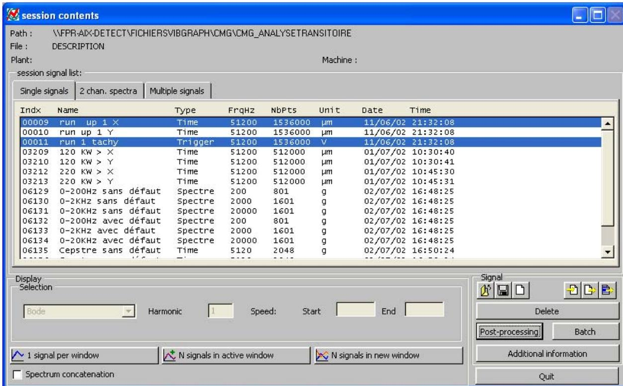
This processing performs, from a Signal item and a Trigger Input item (resulting from the recording of a tachometric transducer on a dynamic channel), an order extraction and yields:
