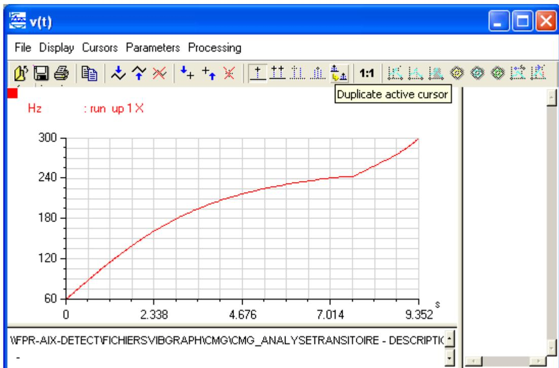
The Speed(t) representation is the plot of rotation speed during a run-up/coast-down phase versus time. It is used to assess a machine's deceleration times, these being characteristic of inner friction.
