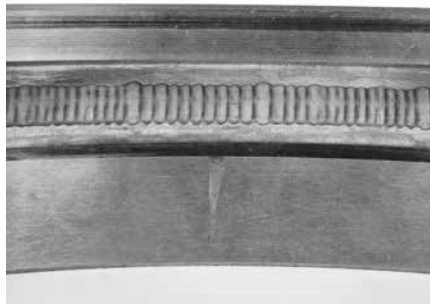
Burns from electric current.
