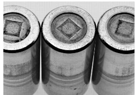
Scoring damage on roller end.
