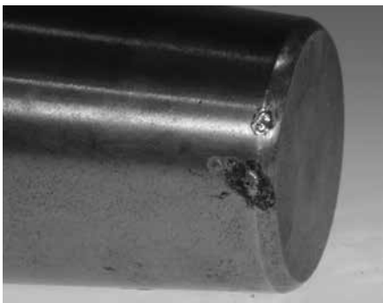
Roller with electric arc burns.
