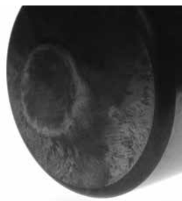
Roller end with adhesive wear.
