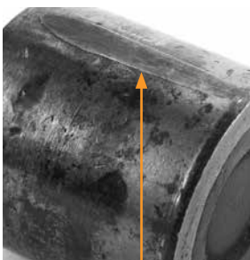
Roller flats, adhesive and skidding wear on raceway surface.
