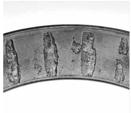
Advanced spalling initiated at water etch marks on the outer ring race makes this bearing unsuitable for further service.
