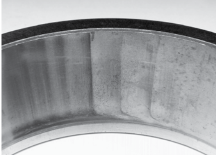
Scalloping marks in the outer ring are common with excessive endplay. This occurs when unloaded rollers enter the small load zone and are suddenly exposed to heavy loads.
