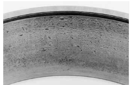
Debris from other fatigued parts, inadequate sealing or poor maintenance caused bruising on this tapered roller bearing race.
