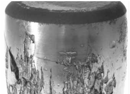
Heavy spalling and fracturing from high loads on this spherical roller bearing.
