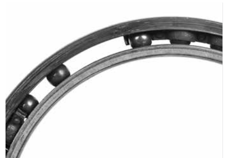
Cage damage from bearing lockup.
