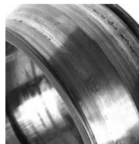
Adhesive wear on bearing inner ring.
