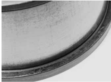
Rib and roller end heat damage.
