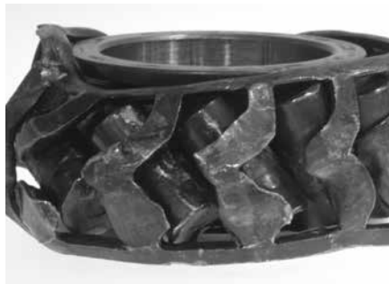
Cage damage from bearing lockup.
