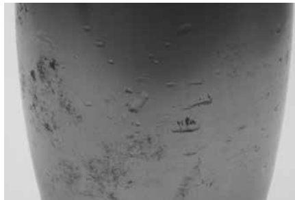
Hard particles caused contamination bruising on this spherical roller bearing.
