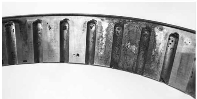
Heavy false brinell on outer race.
