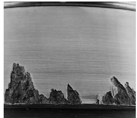
Geometric Stress Concentration (GSC) spalling.
