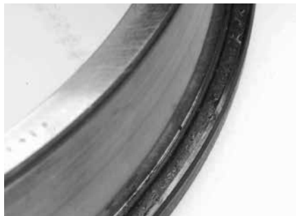
Level 2 – Advanced rib scoring is due to inadequate lubricant film.
