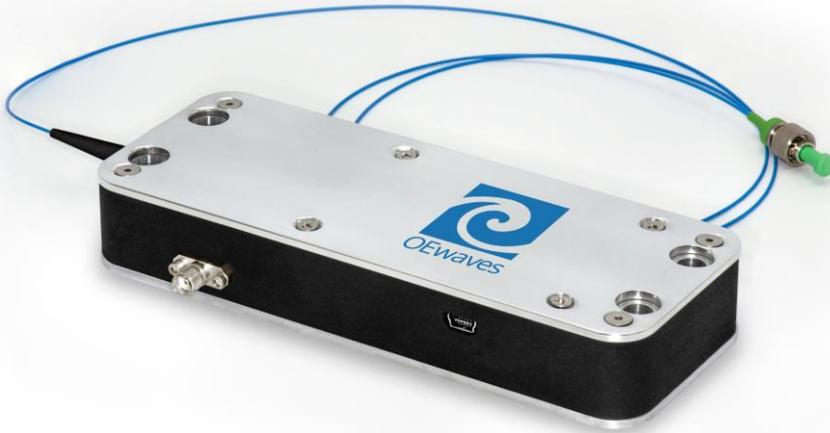
This HI-Q™ Laser houses a proprietary driver/controller and the OEwaves laser source which is based on a high quality factor (Q) Whispering Gallery Mode (WGM) micro-resonator. The laser is available at a variety of wavelengths within 980 – 1080 nm.
