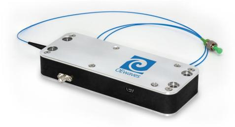
This HI-Q<sup>™</sup> laser houses a proprietary driver/controller and the OEwaves laser source which is based on a high quality factor (Q) Whispering Gallery Mode (WGM) micro-resonator. The laser is available at a variety of C band wavelengths (1530 – 1565 nm).
