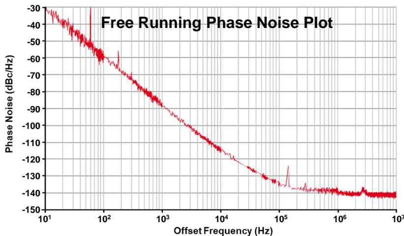
HI-Q™ Nano OEO offers phase noise performance better than -110 dBc / Hz at 10 kHz off set from the carrier.
