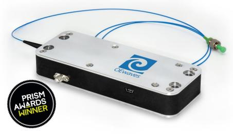
This HI-Q<sup>™</sup> laser houses a proprietary driver/controller and the OEwaves laser source which is based on a high quality factor (Q) Whispering Gallery Mode (WGM) micro-resonator. The laser is available at a variety of C band wavelengths (1530 – 1565 nm).
