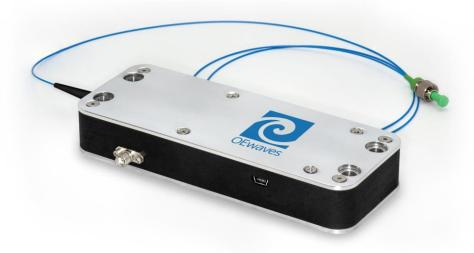
This HI-Q<sup>™</sup> laser houses a proprietary driver/controller and the OEwaves laser source which is based on a high quality factor (Q) Whispering Gallery Mode (WGM) micro-resonator. The laser is available at a variety of C band wavelengths (1530 – 1565 nm).
