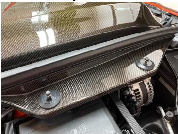
2. Remove the factory engine cover mounting brackets
