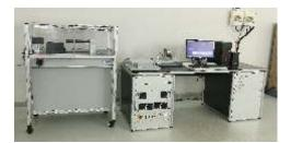
Epstein frame with stator core tester
