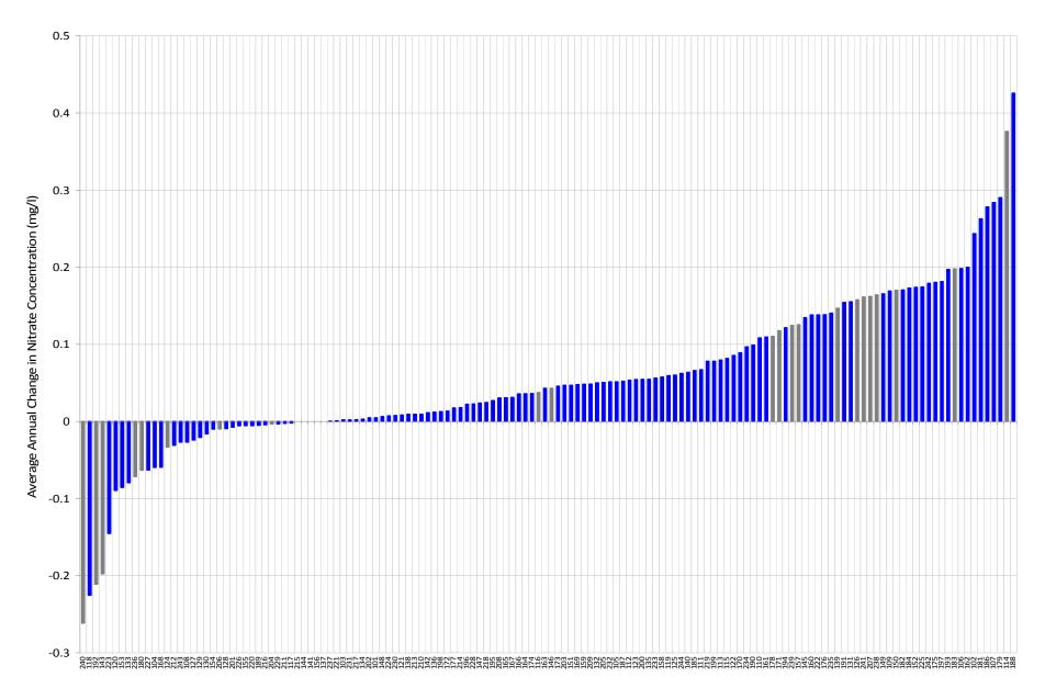
Figure 8. Bar graph depicting nitrate trends at Hillside private wells with 4 or more tests. Individual plots are provided in Appendix A and locations of systems are shown on figure 10 using the well number shown.
