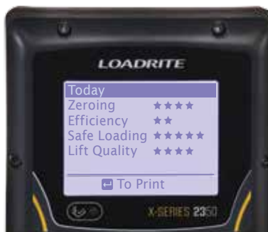
Operators are given a rating to quickly understand performance
