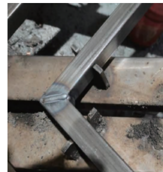
0.8mm Plate Welding ◀
