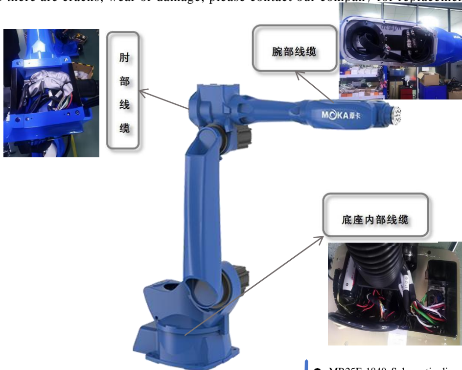
● MR25E-1840 Schematic diagram of robot cable layout
