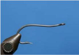
1. Bend down the hook barb. Bend hook shank up about 10-15 degrees  $\frac{1}{4}$ " behind eye of hook (see photo). A simple way to bend the hook is to hold it securely with needle nose pliers at the  $\frac{1}{4}$ " point and then apply upward pressure on rear of hook with fingers.
