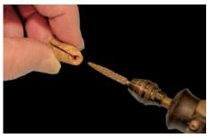
8. Back-drill the hole in the small end of the popper for the hook dressing. Use a small drill or a small tapered burr.
