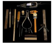
1. Here are the tools we need: A Dremel Tool, center finder rule, headless deck screw, small rasp, fine toothed hack saw blade, small fine toothed round and tapered burrs (Kutzall), a caliper (preferably dial), small cut-off wheel, some sand paper, paint and Sparkle paste.
