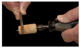
3. Brace the Dremel Tool on the edge of a waste basket and running the tool at about half speed lightly press the small rasp to the cork and slowly shape the cork body. This goes very quickly so be a careful not to take off too much cork. Sand the body smooth finishing with 180 and 220 grit paper. Check the front and rear diameters with the caliper. When you have the shape you want, remove the cork from the screw and prepare to make the hook slot.
