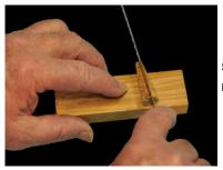
5. Mark the body and cut the hook slot with the fine tooth hack saw blade using a pull motion rather than pushing the blade: It is easier and more accurate.
