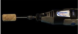
2. Using a center-finder rule, locate the center point of the end of the cork. Take an ice pick and press it as straight as you can all the way into the cork. This makes a path for the screw. With the screw mounted in the Dremel Tool, thread the cork on the screw all the way to the tool chuck.
