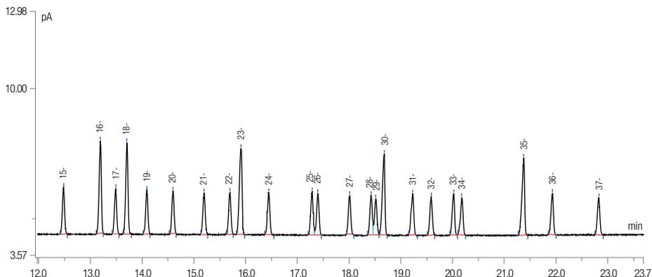
**Figure 6c (peaks 15–37). Analysis on a TRACE TR-FAME GC column 10 m × 0.10 mm × 0.2 μm cyanopropyl phase using nitrogen carrier gas. (Experiment 3)**
