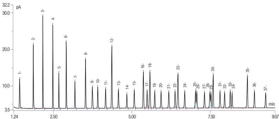
**Figure 4a (full chromatogram hydrogen).** Fast analysis on a TRACE TR-FAME GC column 10 m × 0.10 mm × 0.2 μm with Hydrogen carrier gas. (Experiment 2)
