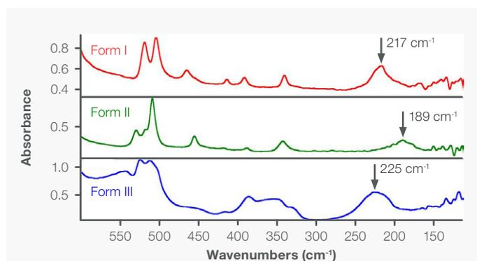
Figure 5. Far-IR transmission spectra of Forms I, II, and III of acetaminophen on PE IR cards.
