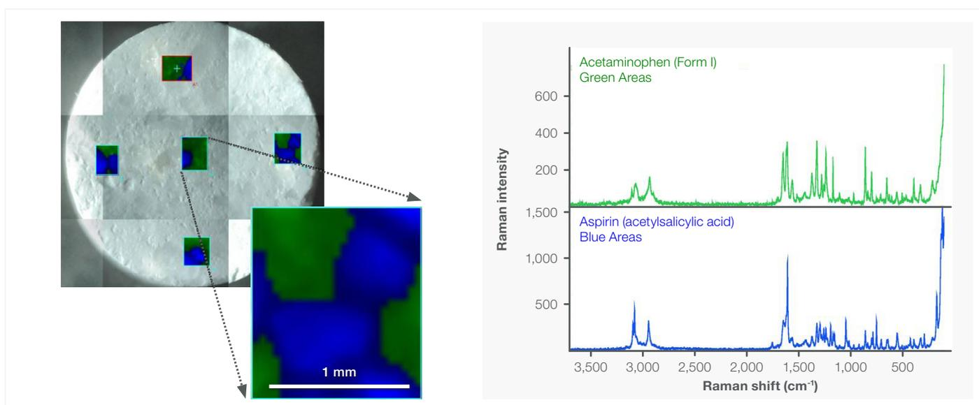
Figure 10. FT-Raman mapping of 5 regions on a commercially available migraine tablet. The MCR images show the distribution of the two largest components (acetaminophen – Form I (green) and aspirin (blue)).
