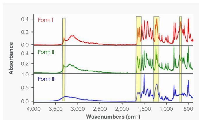
**Figure 2. Mid-IR diamond ATR spectra of Forms I, II, and III. The regions highlighted in yellow show the difference between the spectra.**
