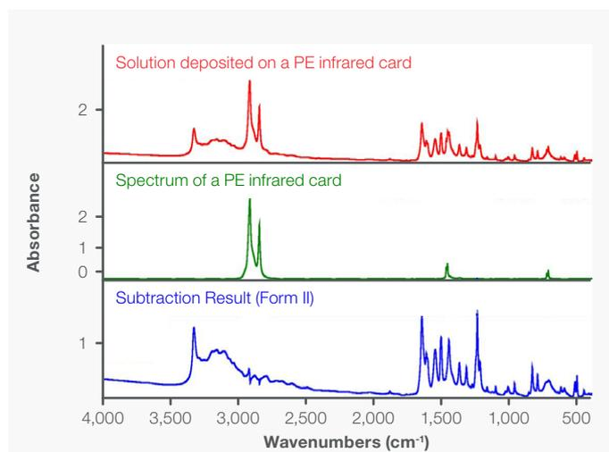
Figure 3. Mid-IR transmission spectra for a methanol solution of acetaminophen deposited on a PE IR card, a blank PE card, and the subtraction result (Form II).
