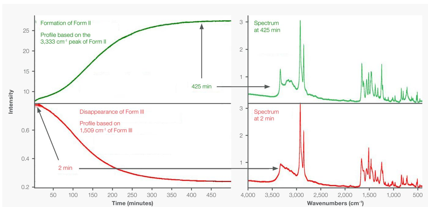
Figure 4. Times series peak area profiles showing the transformation of Form III to Form II for material deposited on a PE Card. Spectra are from 2 minutes (Form III) and 425 minutes (Form II).
