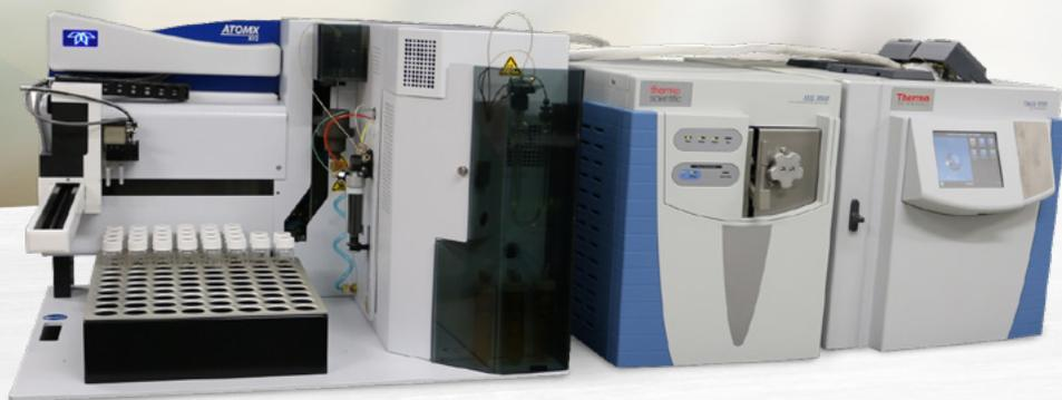
**Teledyne Tekmar Atomx XYZ P&T coupled with the ISQ 7000 single quadrupole MS system and the TRACE 1310 Gas Chromatograph**
