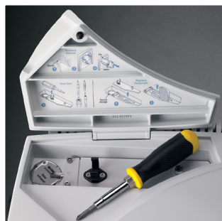
Optional tungsten halogen source and desiccant cartridge are easily accessible
