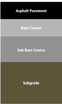
would make for a very weak, easily destroyed road. On good, solid ground, however, it is not uncommon to lay only a surface, binder and base course, and skip the sub-base as the existing soil can take the loading directly from the base course. Older roads may have skipped the base and sub-base courses entirely and simply are a layer of asphalt on top of the subgrade. Such roads are likely to be very prone to failures and should be replaced as soon as practical.
