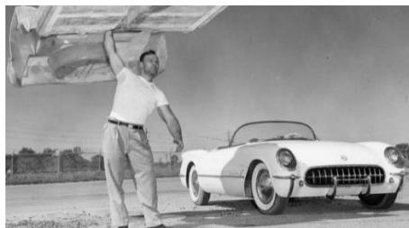
Corvettes weren't supposed to have fiberglass bodies. The original plan was to use steel stamped out on Kirksite dies. But to get that spiffy new Corvette finished in time for the January 1953 Motorama show, Chevrolet had to turn to GRP, which could be churned out way faster.
