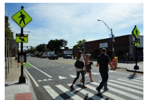
Figure 36: Rectangular Rapid Flash Beacon
