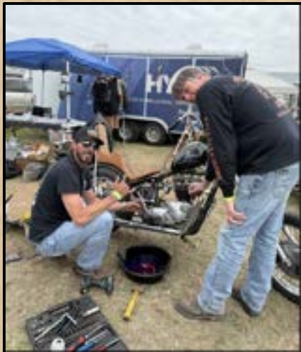
In true swap meet style, Jacob Purty broke down, so we fixed his Triumph. It was stuck in third gear.
