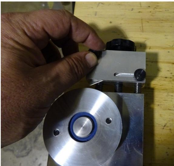
Loosen (2) Blade Cover Screws
