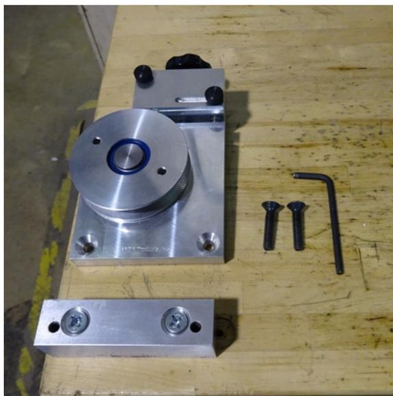
Drill (2) 3/16" holes through your bench using the center (2) holes on the Universal Mounting Bracket as a guide. Screw the bracket down to your bench using the (2) 1/4" wood screws that come with the kit. If your screwing into a hardwood bench applying soap to the threads of the screw makes it easier to tighten completely.
