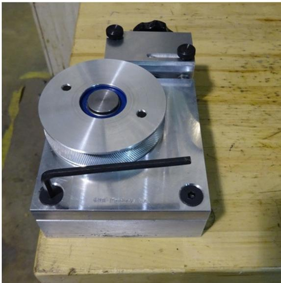
Tighten the (2) 1/4" -20 flathead machine screws with a 5/32" allen wrench.
