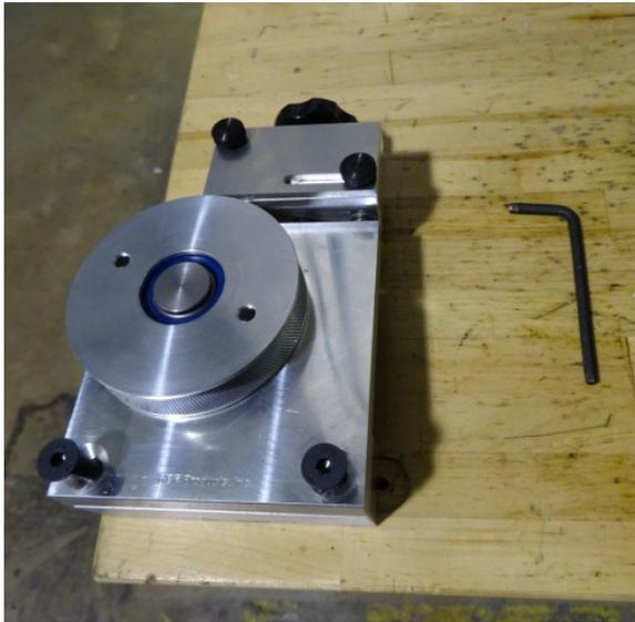
Align the (2) countersunk holes in the stripper frame up with the (2) outer tapped holes of the Universal Mounting Bracket. Thread the (2) 1/4" - 20 Flathead machine screws into the bracket.
