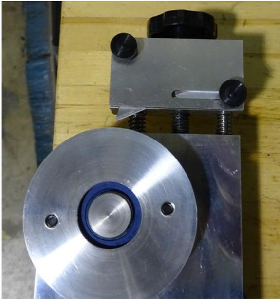
Slide the Blade Cover back over the Blade and tighten the Blade Cover Screws.
