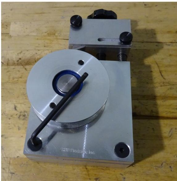
Tighten the 1/4" - 20 flathead machine screws with a 5/32" allen wrench.
