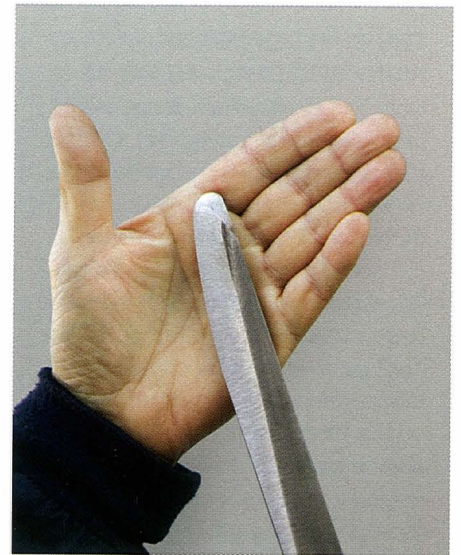
A narrow blade like on this negative-rake scraper is ideally suited to turn tall, narrow exotic bowls. The negative-rake angle is first ground on the 10V steel so the tool can be touched up many times with a new burr before requiring you to grind the negative angle again.
