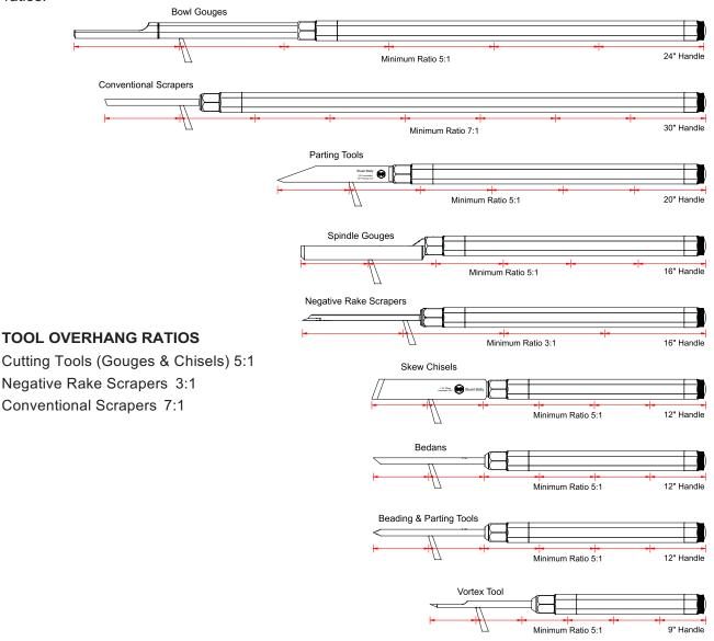
Understanding overhang ratios is an essential aspect of woodturning. Using the correct ratio for each group of tools will reduce fatigue and enable much better stable tool control.
