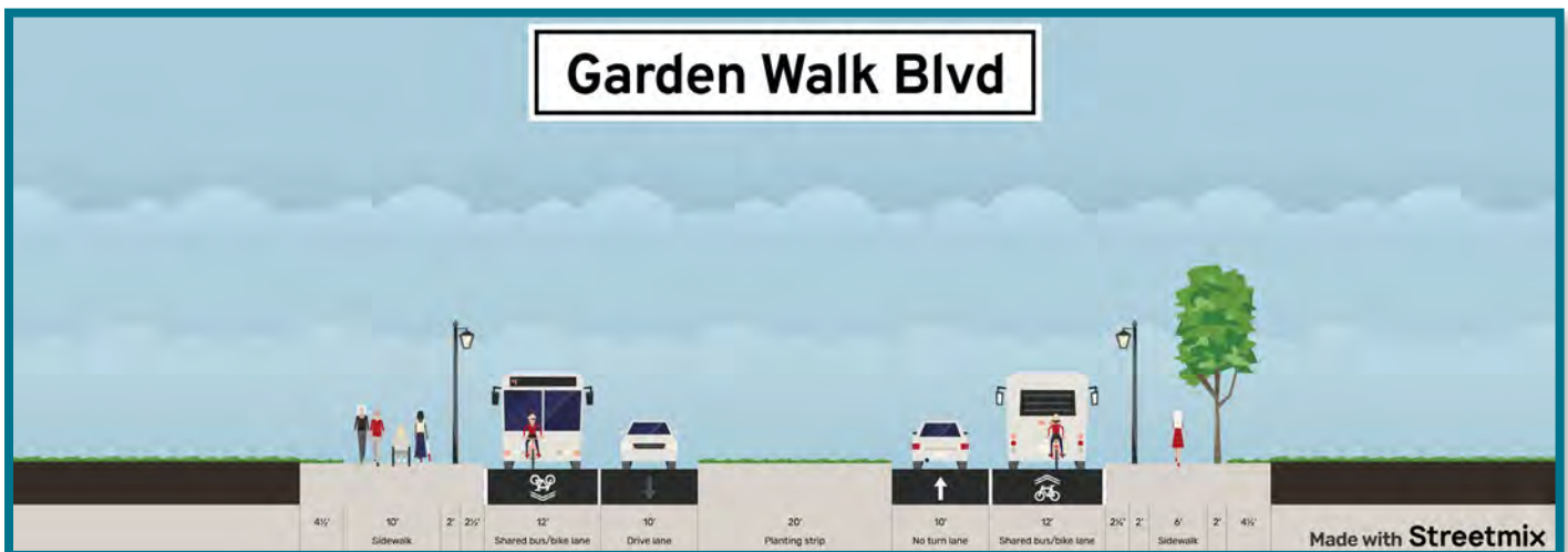
Figure 5-18: Garden Walk Boulevard Roadway Section Concept
