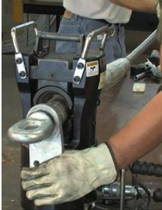
After the entire dead-end body is completely pressed on to the 3M ACCR, take care to secure the dead-end assembly to the rigging and do not allow the dead end to be dropped.
