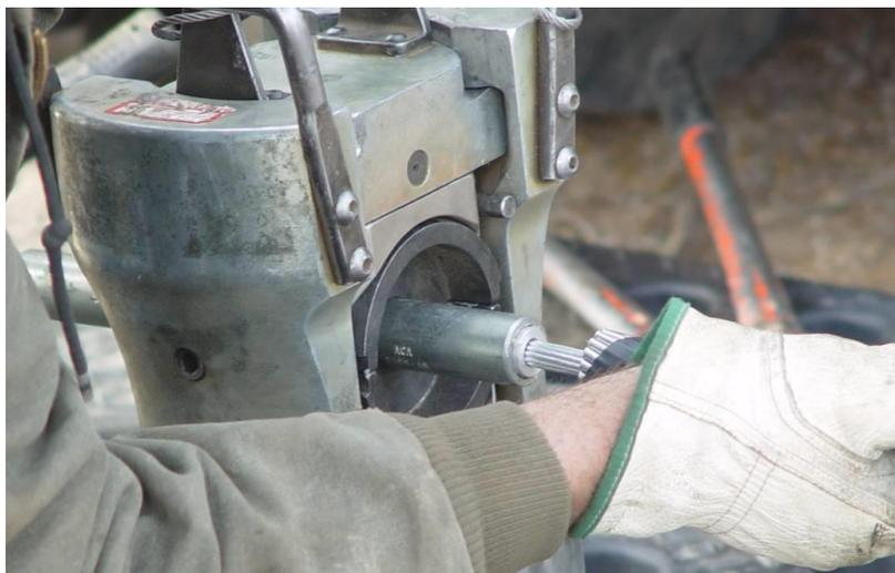
Continue to press the entire length of the steel forging from the first compression bite at the center towards each end of the steel forging, overlapping each die bite by 0.5” (10mm). Lubrication of the steel forging is not recommended.
