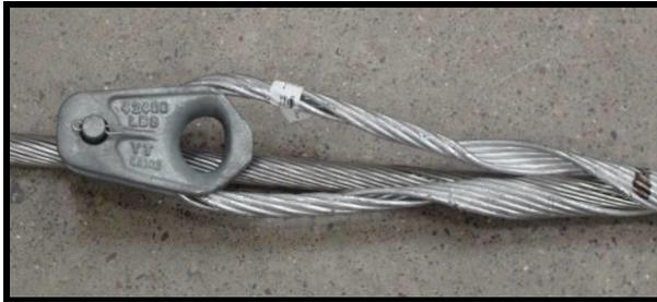
**Thimble Clevis installed on TG-Grip**
