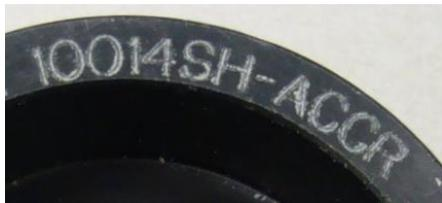
All qualified “-ACCR” stamped dies may be purchased through 3M. Any dies not stamped may be sent to 3M to be measured, qualified and then stamped with the “-ACCR” suffix. Please contact 3M for more information on where to ship your dies to be qualified for usage when installing compression hardware on the 3M ACCR.
