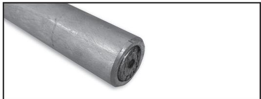
**Step #5** Apply the supplied oxide inhibitor to the non-tapered portion of the aluminum inner sleeve.
