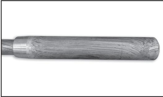
**Step #6** Slide the jumper onto the inner aluminum sleeve such that 1" of the inner aluminum sleeve is sticking out.
