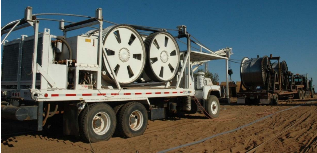
Figure 8. Dual drum bullwheel, courtesy of Oncor.
