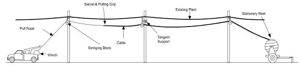
Figure 1 - Stationary Reel Method of Cable Deployment
