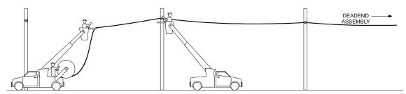
Figure 4 - Drive Off Method of Cable Deployment
