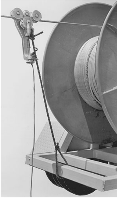
Figure 13.6 A running ground connection is designed to keep the conductor grounded as stringing operations are in process. A rope is used to secure the connector in place. (Courtesy of Sherman & Reilly, Inc.)
