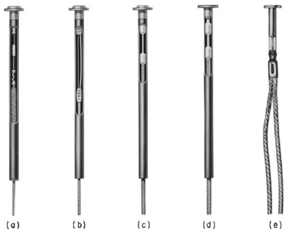
Figure 8.2 These primary cutout fuse links have different fusible elements. (a) a high-surge dual element (1 to 8 amps); (b) a wire element (5 to 20 amps); (c) a die-cast tin element (25 to 50 amps); (d) a die-cast tin element (65 to 100 amps); and (e) a formed strip element (140 to 200 amps).
