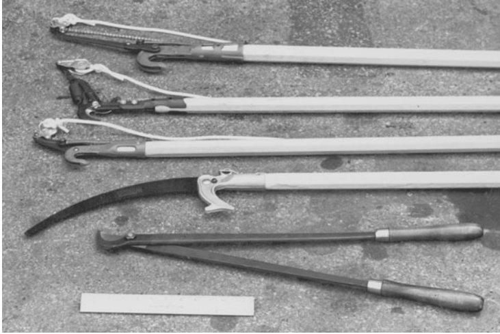
Figure 10.4 Trimming hand tools. Starting at the top, tools are a center-cut bull clip, a side-cut pole clip, a center-cut pole clip, a pole saw, and a pair of loppers. (Courtesy of Asplundh Tree Expert Co.)
