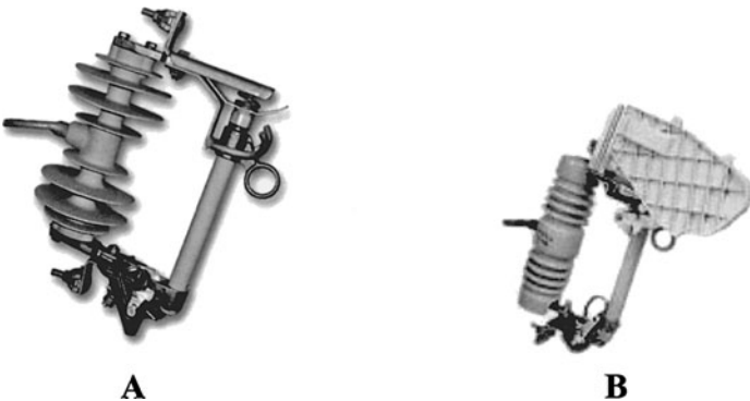
Figure 8.5 (A) Distribution cutout with expulsion fuse mounted. The fuse is in the closed position, completing circuit between top and bottom terminals. (B) Open distribution cutout with arc chute designed for load break operation. (Courtesy of ABB Power T&D Company Inc.)
