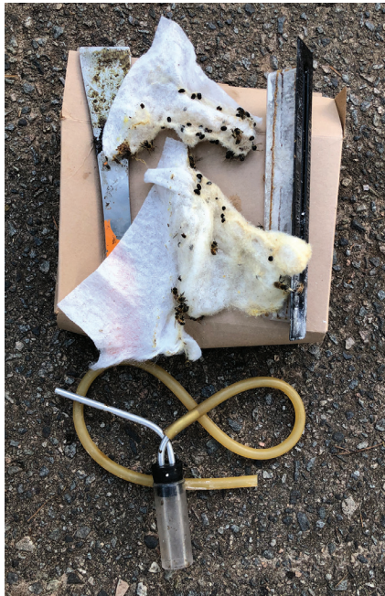
The aspirator is the piece of equipment with the yellow hose. The hose goes to the mouth and the exposed metal tube collects the beetles. The beetles are trapped in a clear container.
