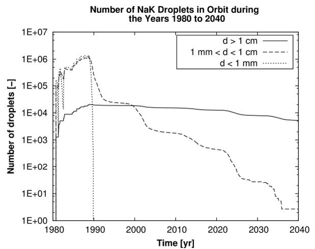
Figure 3. Simulated evolution of the number of NaK droplets in orbit
