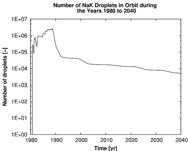
Figure 2. Simulated evolution of the number of NaK droplets in orbit
