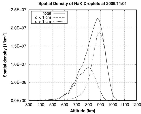
Figure 7. Spatial density of NaK droplets for two diameter classes in 2009
