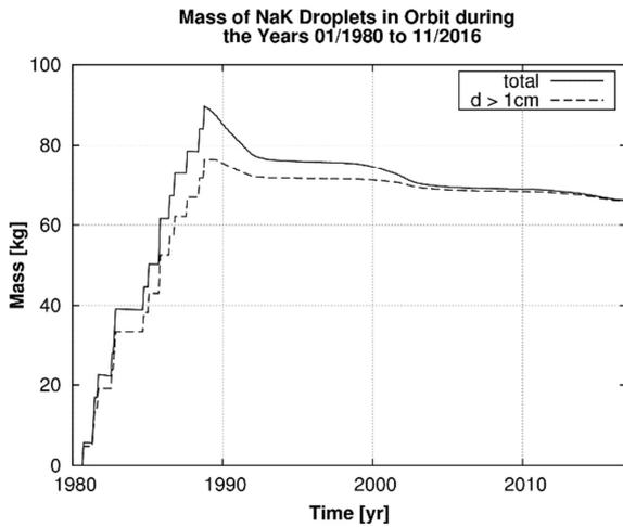
Figure 1. Simulated mass of NaK droplets in orbit
