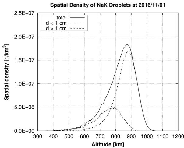
Figure 8. Spatial density of NaK droplets for two diameter classes in 2016
