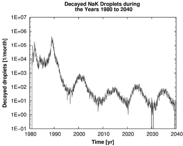
Figure 4. Simulated decay behaviour of NaK droplets shown as monthly decayed number of objects
