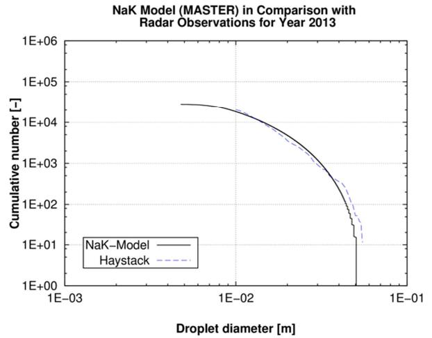
Figure 6. Comparison of the NaK size distribution model with radar measurement data taken from Krisko et al. (s. Fig. IV in [25])
