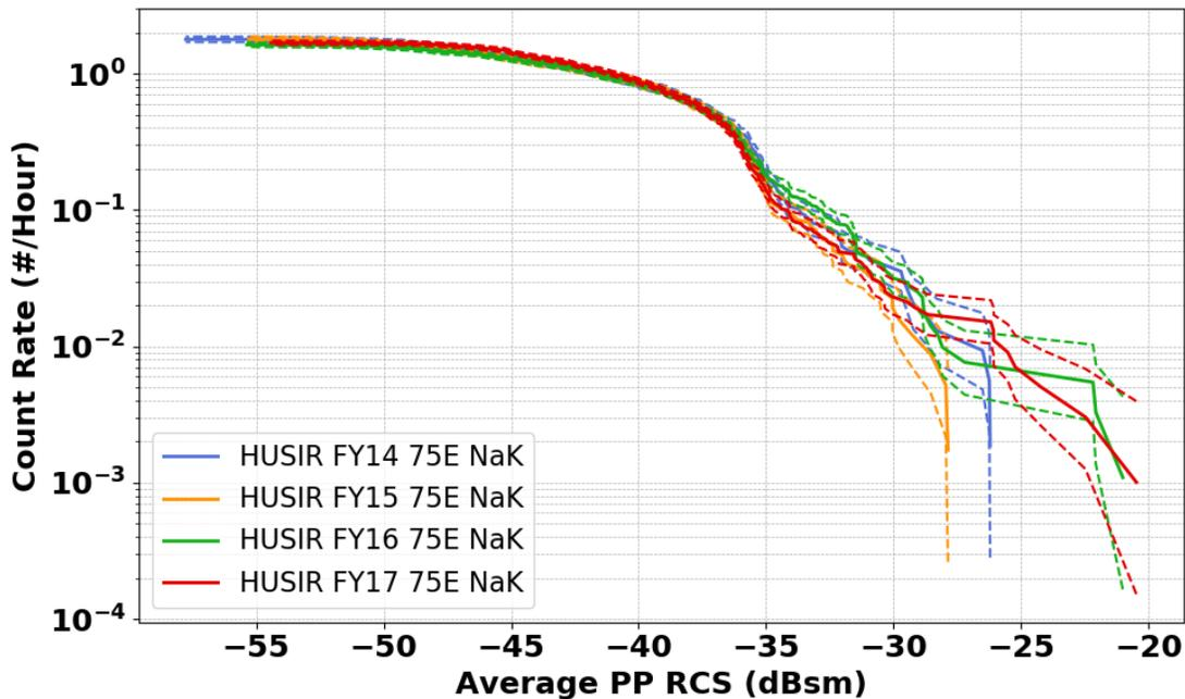
Figure 4-6. PP RCS Cumulative Distribution of the NaK population extracted from all 75° elevation data by year.
