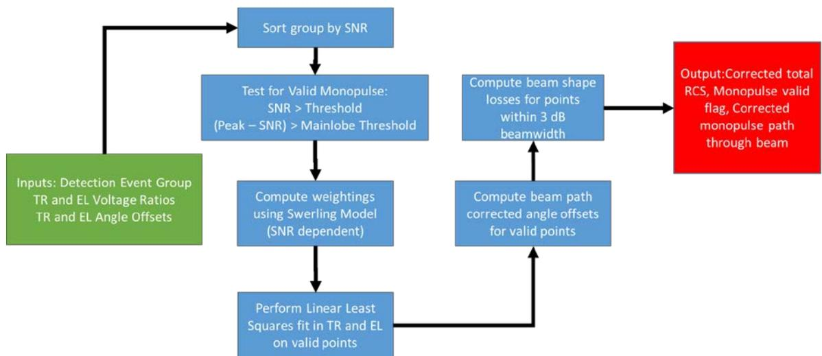
Figure 3-9. Algorithm for estimating monopulse-derived path through the beam.
