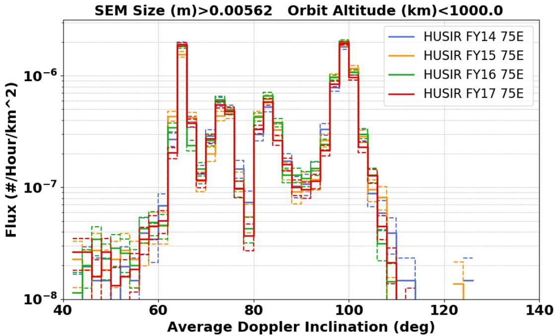
Figure 4-10. Cumulative surface area flux versus altitude limited to 5.62 mm for all 75° elevation data by year. The dashed lines represent 1σ uncertainty bounds.
