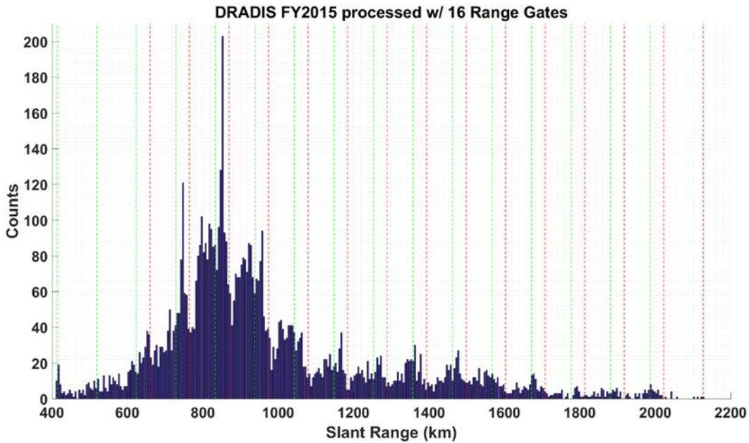
Figure 3-13. Counts versus slant range with 10 km bins for 16 range gates. The green and red vertical lines correspond with the start and stop ranges, respectively, of each range gate. The spikes in detections correspond with overlap between range gates.
