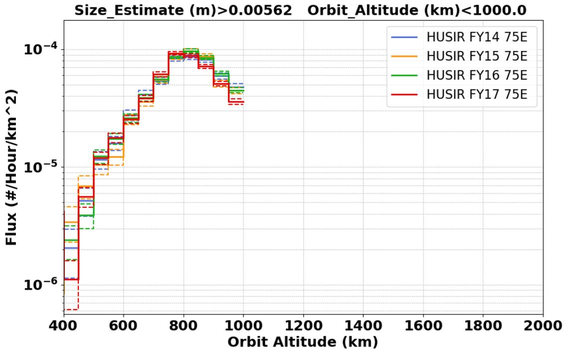
Figure 4-8: Cumulative surface area flux versus altitude limited to 5.62 mm for all 75° elevation data by year. The dashed lines represent 1 $\sigma$  uncertainty bounds.
