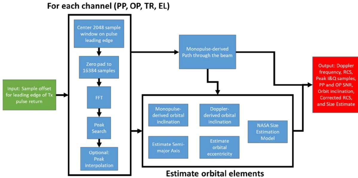
Figure 3-8. Second measurement pass algorithm conducted by DRADIS.
