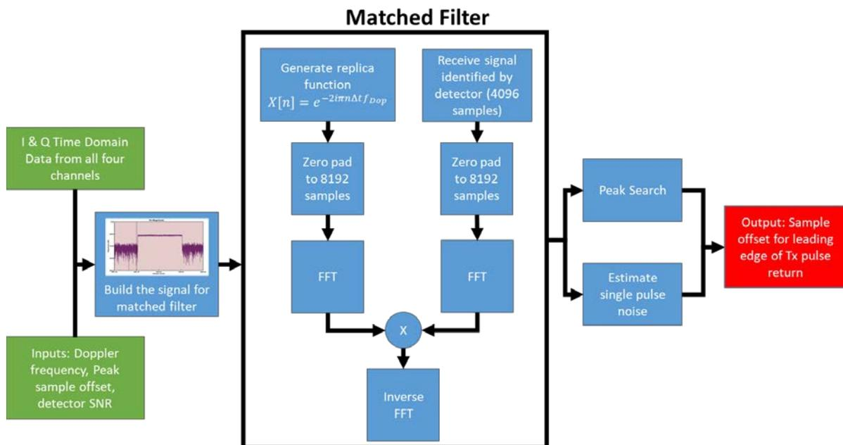
Figure 3-7. First measurement pass algorithm employed by DRADIS.
