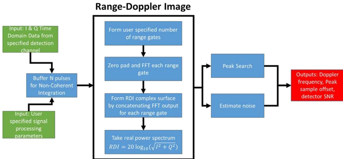
Figure 3-6. Detection pass algorithm employed by DRADIS.
