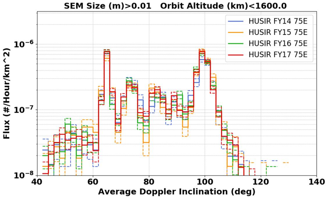
Figure 4-9. Cumulative surface area flux versus inclination limited to 1 cm for all 75° elevation data by year. The dashed lines represent 1σ uncertainty bounds.
