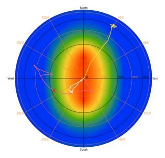
If only one well is displayed the Well trajectory is coloured blue to red with increasing depth for a single trajectory. Well trajectories for multiple wells will be coloured according to their assigned colour in trajectory table on the Display Options tab.
