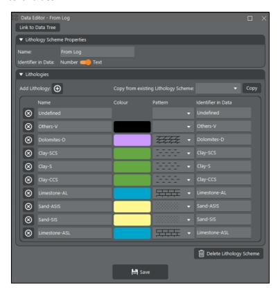
The Log Editor has an option to generate a Lithology Scheme from text-based lithology logs (discrete or segment). Unique identifiers from lithology log values are automatically assigned a colour and pattern by parsing the identifier labels for recognised names (sand, shale etc).
