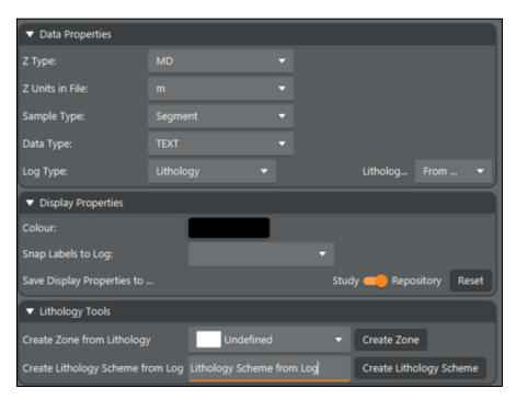
Added the option to define Lithology Schemes from text which can then be applied to discrete or segment-based lithology logs that contain text values.
