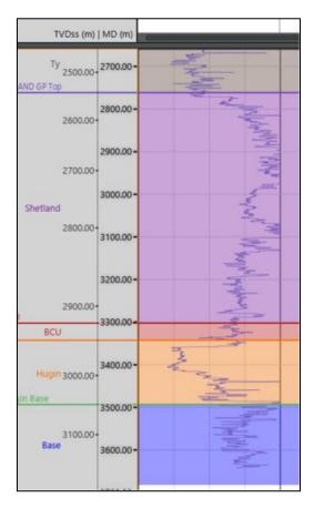
Added ability to apply colour bars to Log Fills. Colour is distributed via the scale of the log being filled. Fills are coloured based on their width.
