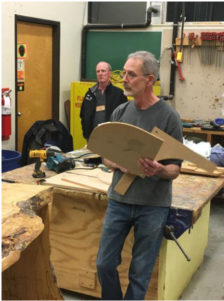
A few of the jigs and templates Jim brought to show and demonstrate how he makes tight fitting curved components
