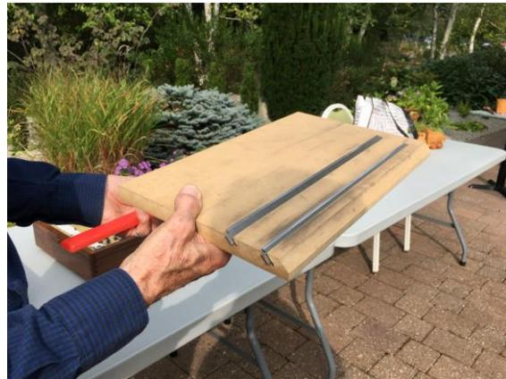
Bruce demonstrated a jig he made of MDF to hold his planer blades for honing. Different depths of each groove produce the desired angle. He uses a Japanese water stone to achieve the desired sharpness.
