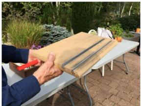
Bruce demonstrated a jig he made of MDF to hold his planer blades for honing. Different depths of each grove produce the desired angle. He uses a Japanese water stone to achieve the desired sharpness.
