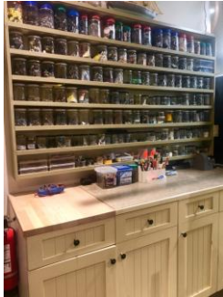
Recycled kitchen cabinets with large mouth jars for small parts storage on shelves above. End wall space utilization. Tooth paste caps for holders instead of peg board.
