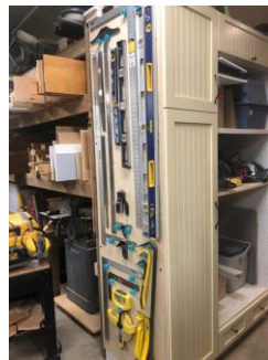
Recycled kitchen cabinets with large mouth jars for small parts storage on shelves above. End wall space utilization. Tooth paste caps for holders instead of peg board.
