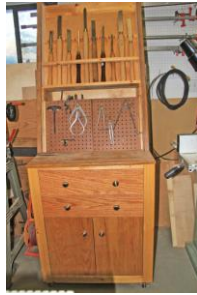
Hinged cabinets for, router & shaper bits, wood lathe tools & accessories, chisels & planes, box parts, etc.
