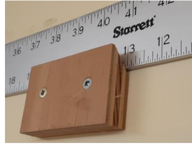
Wall hanger (45° plywood) for clamps, etc.
