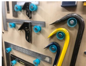
Recycled kitchen cabinets with large mouth jars for small parts storage on shelves above. End wall space utilization. Tooth paste caps for holders instead of peg board.
