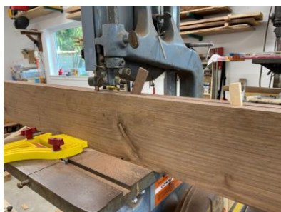
Re-sawing the rails
