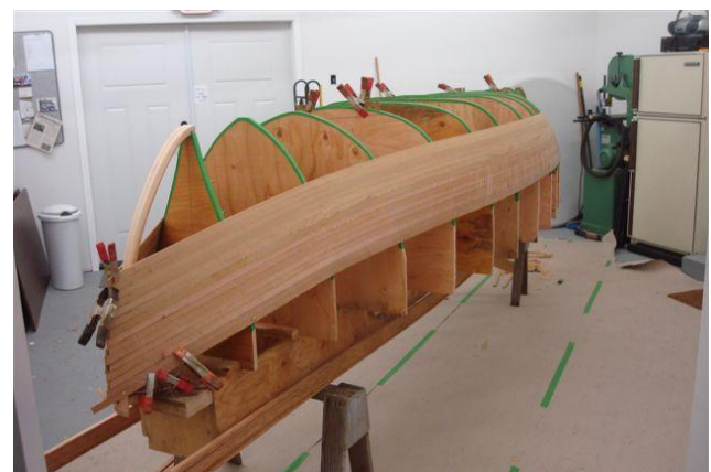
The building form (strong back) and the first four strips on each side. Strips half way up
