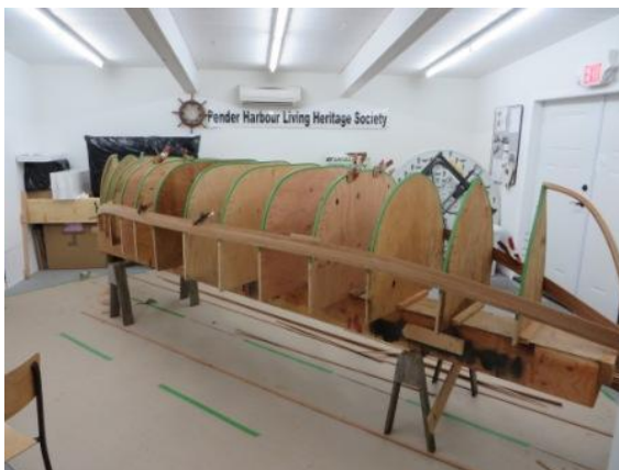
The building form (strong back) and the first four strips on each side. Strips half way up
