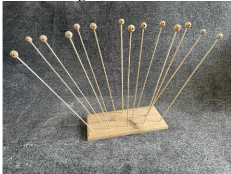
Zip-Lock bag 'drying rack'. Bamboo skewers for the uprights with 5/8" beads for the tips fastened into a cedar base.
