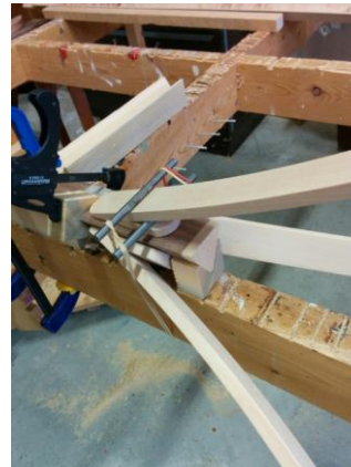
Gluing/fastening legs to the stand
