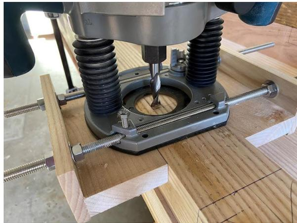
Few of the set-ups and jigs used to cut holes, make mortise & tenons, etc.
