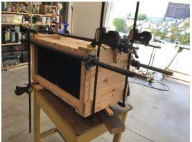
Corners glued together with PL300 and clamped overnight (24 hours).
