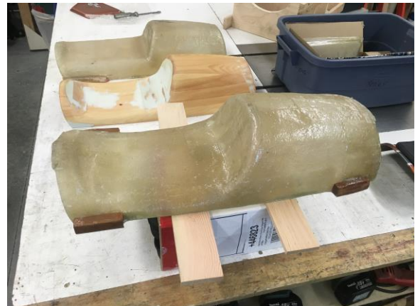
Three parts of the process (front to back). Mould, pattern and unpainted finished fibreglass seat (unpainted).
