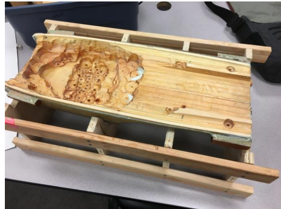
Back (underside) of the pattern hollowed out to reduce weight and check fit on bike.
