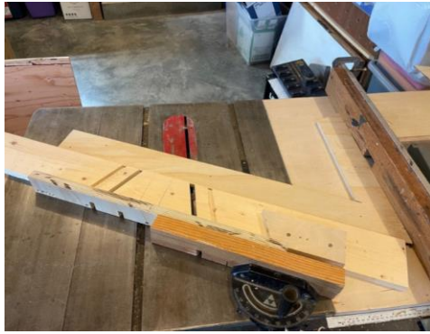
Jig for cutting dados on one leg.
