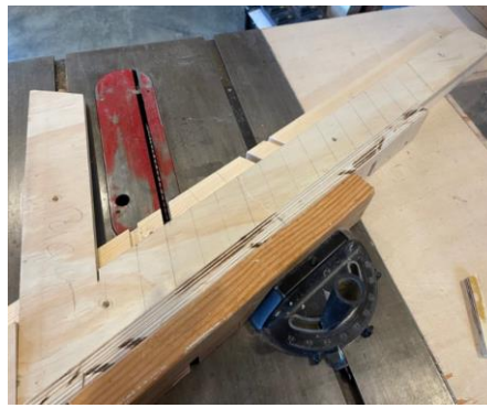
Jig flipped to exactly duplicate dado on other leg.
