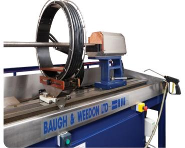
• **Testpiece Supports.** V-block supports are fitted to the head and tailstock as standard. Adjustable support rollers fitted to the head or tailstock, or mounted on the bed bars, can be supplied. A small piece device affords protection to delicate components is also available.
